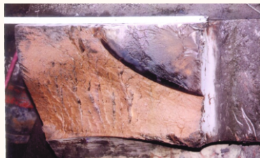
Fig. 3: Fracture face of broken fork
